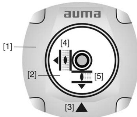
Figure 49: Mechanical position indicator
