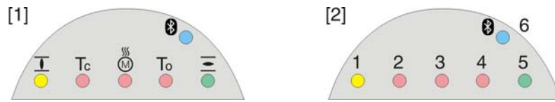
Figure 50: Arrangement and signification of indication lights
