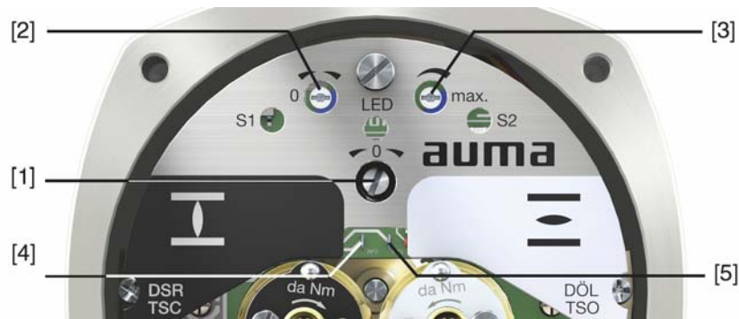
Figure 22: View on control unit when switch compartment is open
